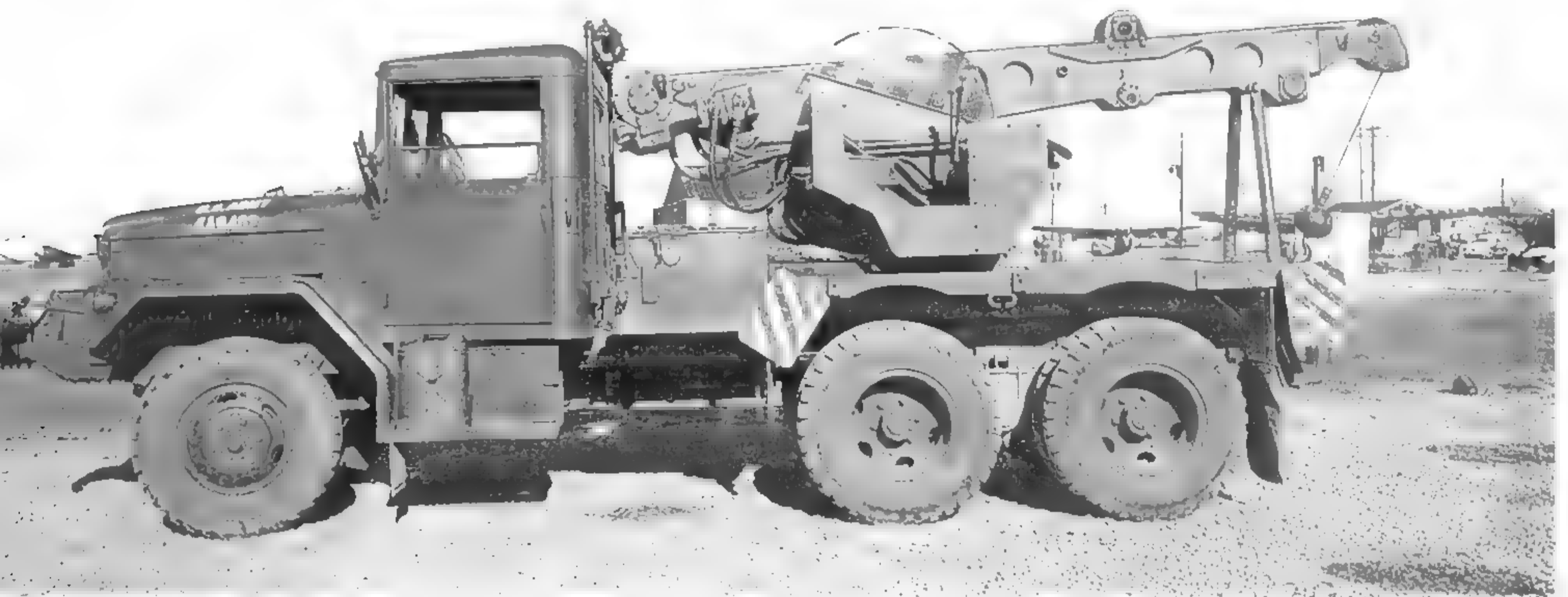
The operator's station of the XM108 was mounted on the side of the boom shipper. It housed controls to maneuver the boom, shipper, and hoist. (Photo courtesy of the Patton Museum)
